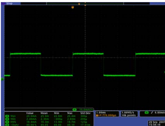
FIGURE 12. I_{LED} AT 50% PWM DIMMING (54 LEDES, 20mA, V_{IN} = 12V )
